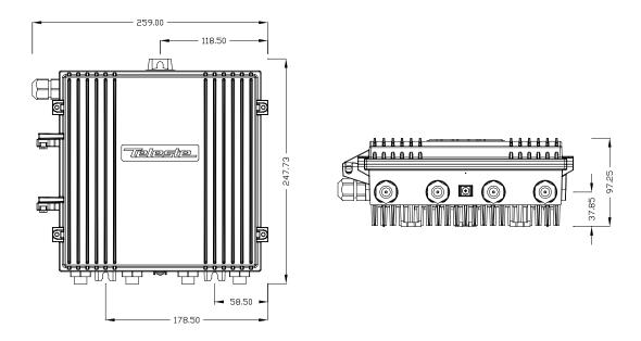
Figure 1. AC3000 housing dimensions - top and side view
