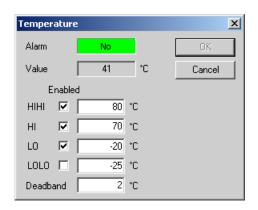
Figure 16. The analog alarm configuration dialog box
