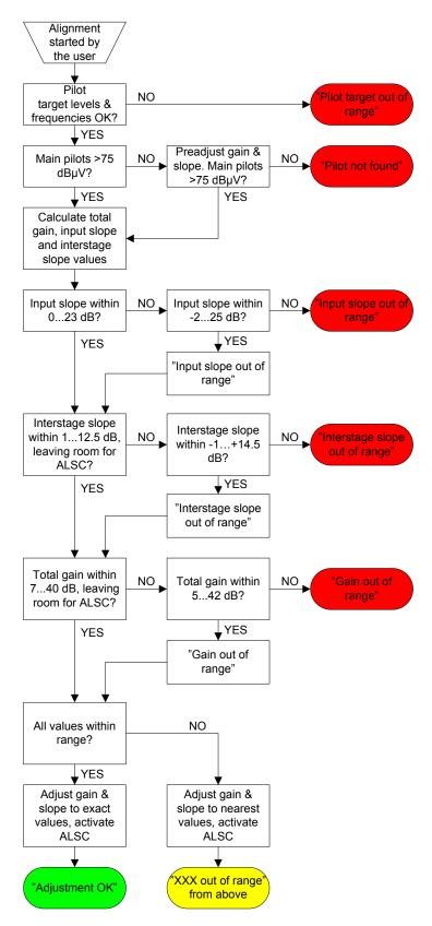
Figure 7. Simplified forward path automatic alignment flowchart
