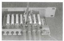
Tighten the ground clip screw until it reaches the bottom. Ensure that there is no foil in contact with the ground clip.
