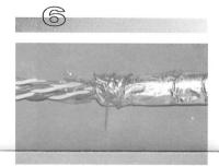
For cable with foil but no braid: Wrap the drain wire around the foil shield. Do not wrap the drain wire more than 1.3 cm (0.5 in.) from the fold in the foil shield. (See instruction 12 for alternative drain wire instruction).
