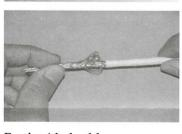
For braided cables: Push the braid back over the jacket of the cable.
