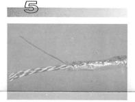
For cable with foil but no braid: Fold the foil shield back over the jacket of the cable.
