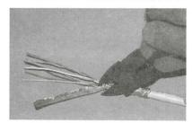
For braided cables: Unwrap the foil that extends beyond the jacket from each pair and cut it off.
