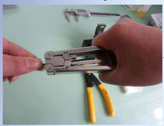
Press and pull out to remove the jacket
