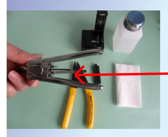
Fix the cable to length 35mm and strip the jacket
