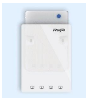
Device Status Lighting is covered by plate
