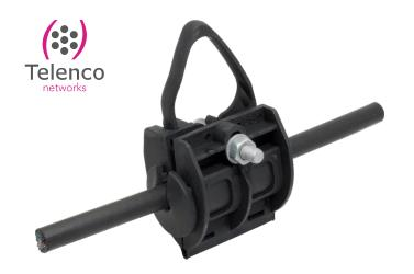
The Telenco® DS suspension clamps are designed to provide a mobile suspension for 5 to 17mm aerial round ADSS cables. These clamps are to install on intermediate poles used for the roll-out of access networks where spans do not exceed 70m.
