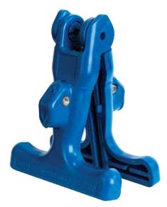
The FOD-2000 puts a slit on both sides of the jacket allowing easy access to the fiber or strength member. The ease of use makes this tool truly unique! To use just position the tool around the cable, pull and slit. A simple twist of the cable allows the jacket and strength members to separate from the buffer tube leaving the fiber undamaged.
