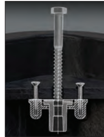
Non-Seizing Bolt System Allows Field Replacement
