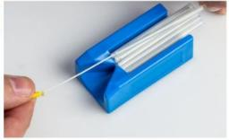
Loading a protection sleeve onto a fiber can be tedious, even for the most experienced technicians. Plus, if they have physical impairments such as poor eyesight then it can become nearly impossible. Designed to make loading protection sleeves onto fiber quick and easy, the QuickSleever protection sleeve insertion tool is ideal for aligning fiber to the holes of protection sleeves and is a real timesaver. This protection sleeve insertion tool features the following:
