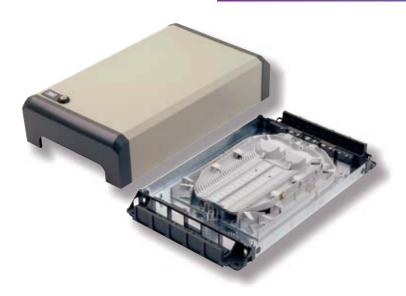
The VKA 8 SCM is an indoor splicing box for building basements. It is the interface between the network and the building distribution. The organiser may be equipped with Evolution trays which are as well designed for fusion & mechanical splices as for splitter integration up to 1x32 PLC splitters.
