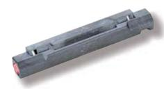
3M Fibrlok 250µm Fibre Splice enables fast, easy splicing of 250µm single-mode fibre in Fibre-to-the-Premises (FTTP) installations. It can also be used in multi-mode LAN installations or any other application where 250µm coated fibre is spliced. This low-loss reliable splice can be installed by non-specialized technicians.
