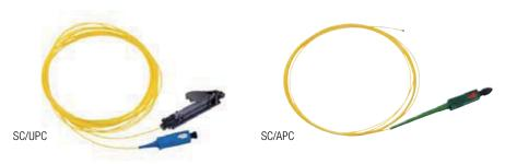
The Fibrlok II splice/holder is also available with a pre-terminated SC/APC or SC/UPC pigtail (0.75 m / 30 inches) for easy installation. Pigtail is fabricated with 10 mm radius, bend insensitive, zero water peak fibre.
