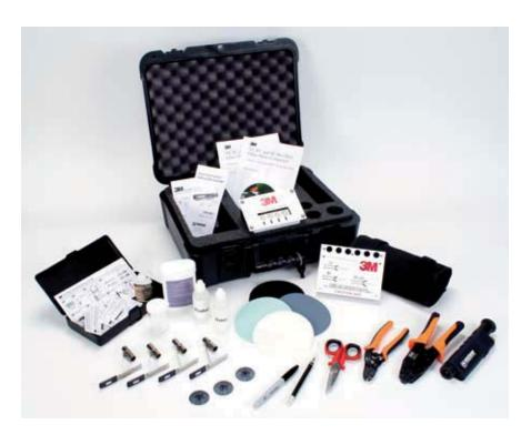
The 3M Hotmelt system offers most convenient field connectivity for fibre optic connectors. From direct termination of breakout cables in patchpanels over pigtails up to patchcords, Hotmelt connectors fit every application. The connectors are pre-filled with Hotmelt adhesive which just needs to be heated for easy termination.
